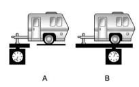
If a weight-carrying hitch or a weight-distributing hitch is being used, the trailer tongue (A) should weigh 10-15 percent of the total loaded trailer weight (B).
